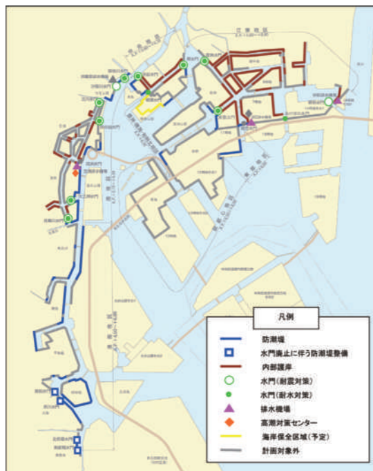
東京港海岸保全施設整備計画図 Facilities Outlined in Port of Tokyo Coastal Protection Facility Preparation Plan
