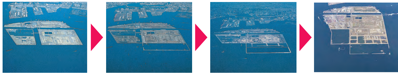
Before construction Shore protection of blocks A & B almost completed Shore protection of block C almost completed Shore protection of blocks G almost completed
