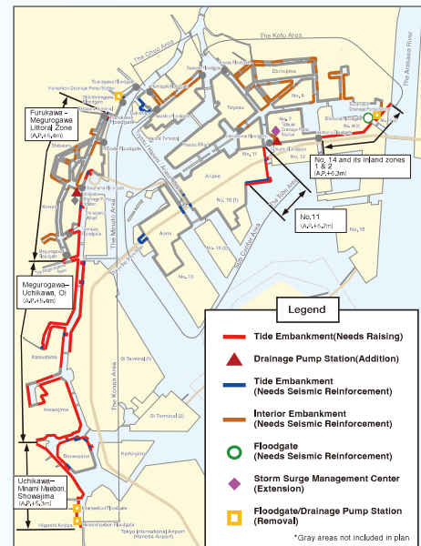
* Drainage pump station installation and positioning in the Koto area TBD
